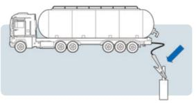
**1.** The truck should be grounded with the appropriate ground cable connection.
