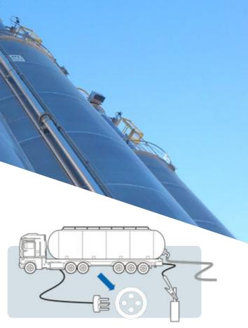
3. Indicate a compatible power outlet to connect the power cord of the truck. Connection to the outlet should be performed by a person qualified for high-voltage work (we recommend the use of LOTO procedures).
